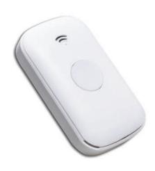
The Q2 is an ideal personal tracker. The Q2 Portable Tracker is a miniature GPS tracker. With alerts like geo-fence boundary crossings, low battery, SIM card change alert and many other advanced reporting features, the Q2 is simply the most versatile tracker. With a 900mAh Li-polymer battery, it is able to work for up to 6 days.
