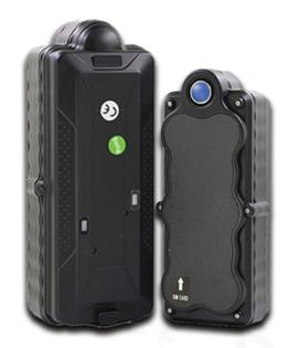
The Trova M2 is a waterproof tracker with 4 built-in magnets. The built-in microphone allows pre-programmed numbers to phone and listen-in. The M2 can be armed so that in idle mode it uses very low power, once movement is detected the unit will activate and begin to track. A programmable panic button on the unit may be used to send a panic and/or call a pre-programmed number.
