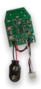
The TX Link is a general purpose transmitter which can be used to interface any device to a radio receiver.
