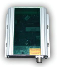
M.A.M.I. VHF radio transmitters are mainly used for alarm panel monitoring and are cable of sending signals up to 40km depending on terrain, this distance can be extended with the use of Repeaters. The signal is typically received on a base station located in a control room connected to alarm monitoring software The VHF radio product range has the following models
