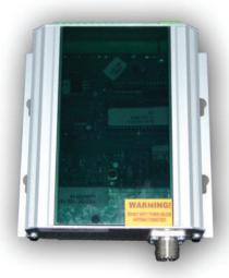
M.A.M.I. VHF radio transmitters are mainly used for alarm panel monitoring and are cable of sending signals up to 40km depending on terrain, this distance can be extended with the use of Repeaters. The signal is typically received on a base station located in a control room connected to alarm monitoring software
