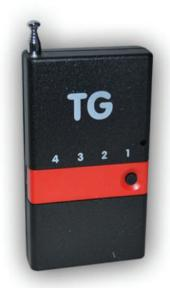
The TG is a 3km FM remote transmitter used in conjunction with a R2/R4 Channel receiver or the versatile RAC receiver. This unit is ideal for panic systems in shopping centers, town house complexes, retirement villages or to control any remote device.
