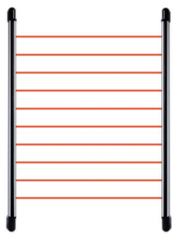
Is a multiple barrier beam comprising an infrared sender and receiver with 6 or 10 active beams. Synchronization is done through a Sync wire or done through the optic beams on the RX and TX. Alarm activation based onDual beam activation, reducing false alarms. Not being able to be cloaked or masked forming an invisible wall rises the level of security. Optional wireless operation with 500m range using localized solar power pack and wireless reporting and control.
