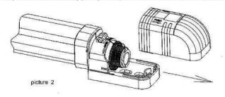
2. Use a 6mm drill bit to make mounting holes in the wall or mounting surface. Insert the plastic masonry plugs into the holes. Use supplied screws or similar, hold the beam in place and screw it to the required surface.
