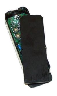
The Gatto is a programmable 2/4 channel receiver capable of storing up to 100 different remote control codes.
