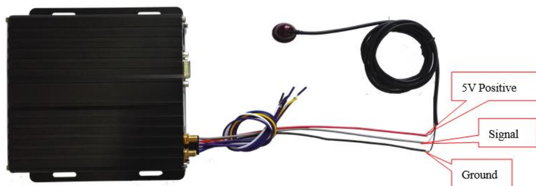
Figure 11. IR extension connection
