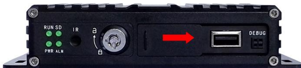
Figure 5. SD card Installation
