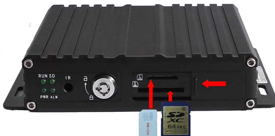
Figure 6. SD card installation
