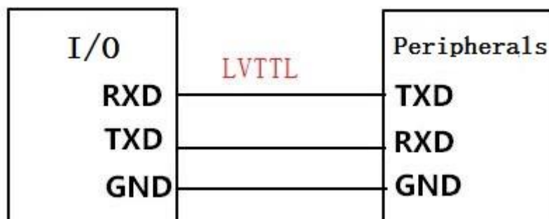
Figure 17. Serial ports Connection
