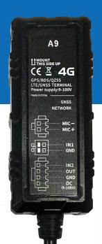
The A9 is a 4G-based IP66 Waterproof LTE GPS tracker. With built-in high-precision GPS positioning module it reports the vehicle location and vehicle status to the vehicle tracking service platform through the 4G network for real-time vehicle monitoring, anti-theft and dispatch management.
